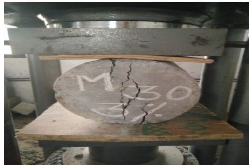
Photo No. 5: Split Tensile Strength Test
