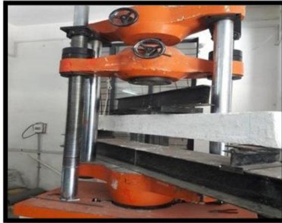
PhotoNo.6: Digital Universal Testing Machine of 100 tones capacity
