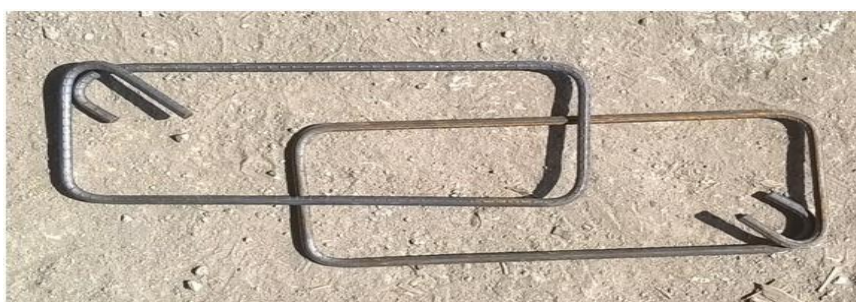
Photo No.3: Reinforcement for Beam Design
