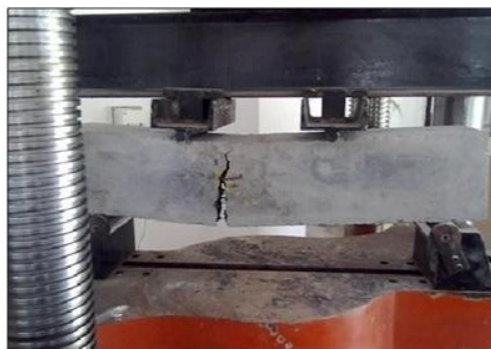
Photo No.7: Failure Pattern of Beam with Steel And Glass Fiber.
