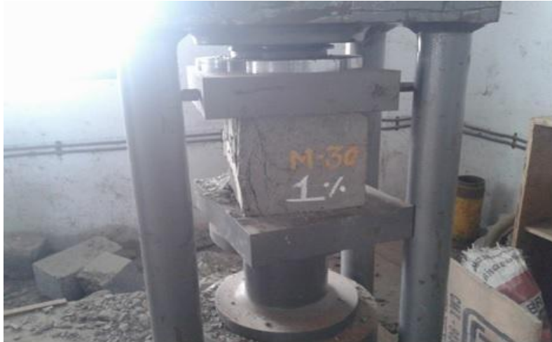
Photo No 4: Testing of cube on CTM
