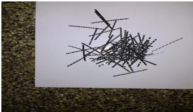
Photo No. 1: Separation of Steel Fibers.
